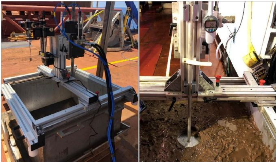
Figure 7.24 Photographs of geotechnical vane and CPT (left) and plate load test (right)
