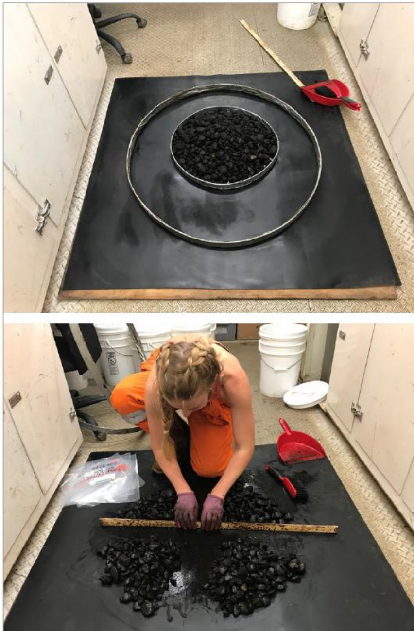
Figure 7.9 Coning and quartering process
