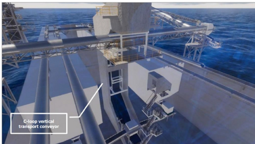
Figure 13.22 Illustration of C-Loop vertical transport conveyor
