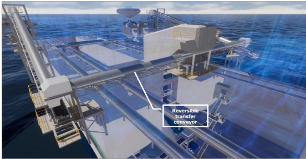
Figure 13.23 Illustration of reversible transfer conveyor
