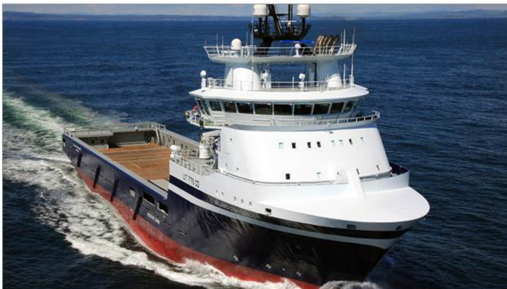
Figure 13.11 MV Island Commander, example of offshore supply vessel used in the oil and gas industry
