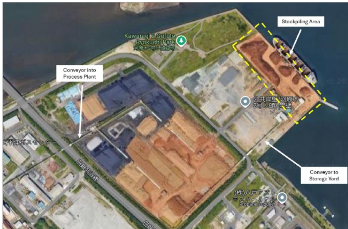
Figure 15.2 Google satellite view of the port unloading area and identification of conveying system used to transport nodules into process plant
