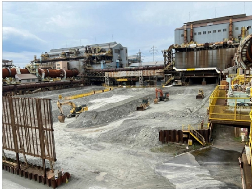
Figure 15.5 PAMCO's slag storage area: slag is left to cool and organized before shipment
