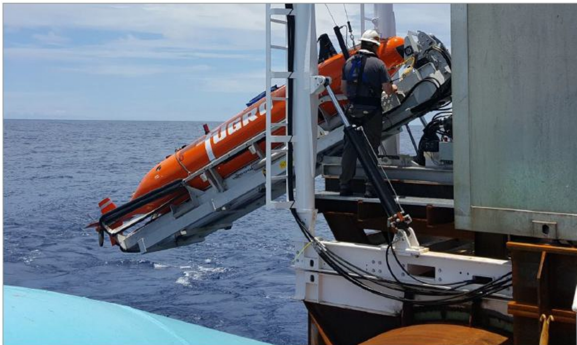
Figure 7.3 Deployment ESVII Kongsberg Hugin AUV from the stern of the Maersk Launcher
