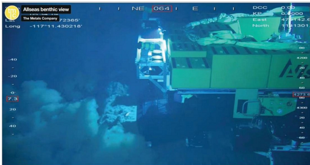
Figure 17.7 Test mining footage showing that the benthic plume stays just above the seafloor
