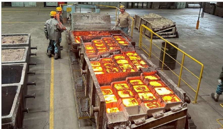
Figure 15.6 Molten alloy tapped into moulds at PAMCO
