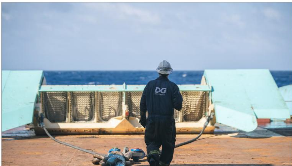
Figure 10.1 Bulk sampling dredge used to collect the bulk sample for metallurgical pilot tests
