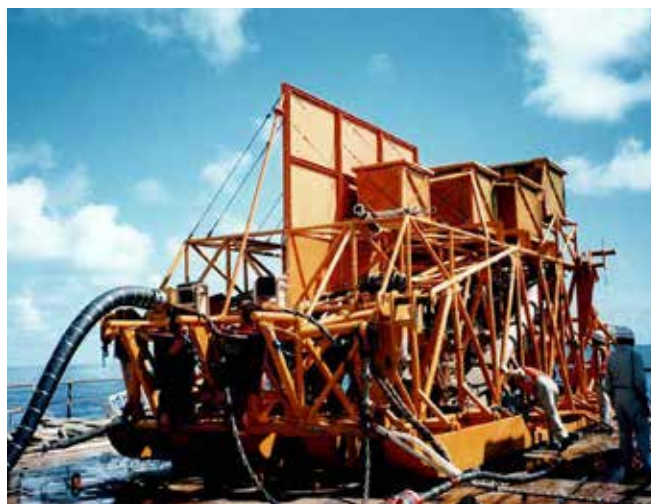
Manganese nodule collector. Photo courtesy COMRA.
