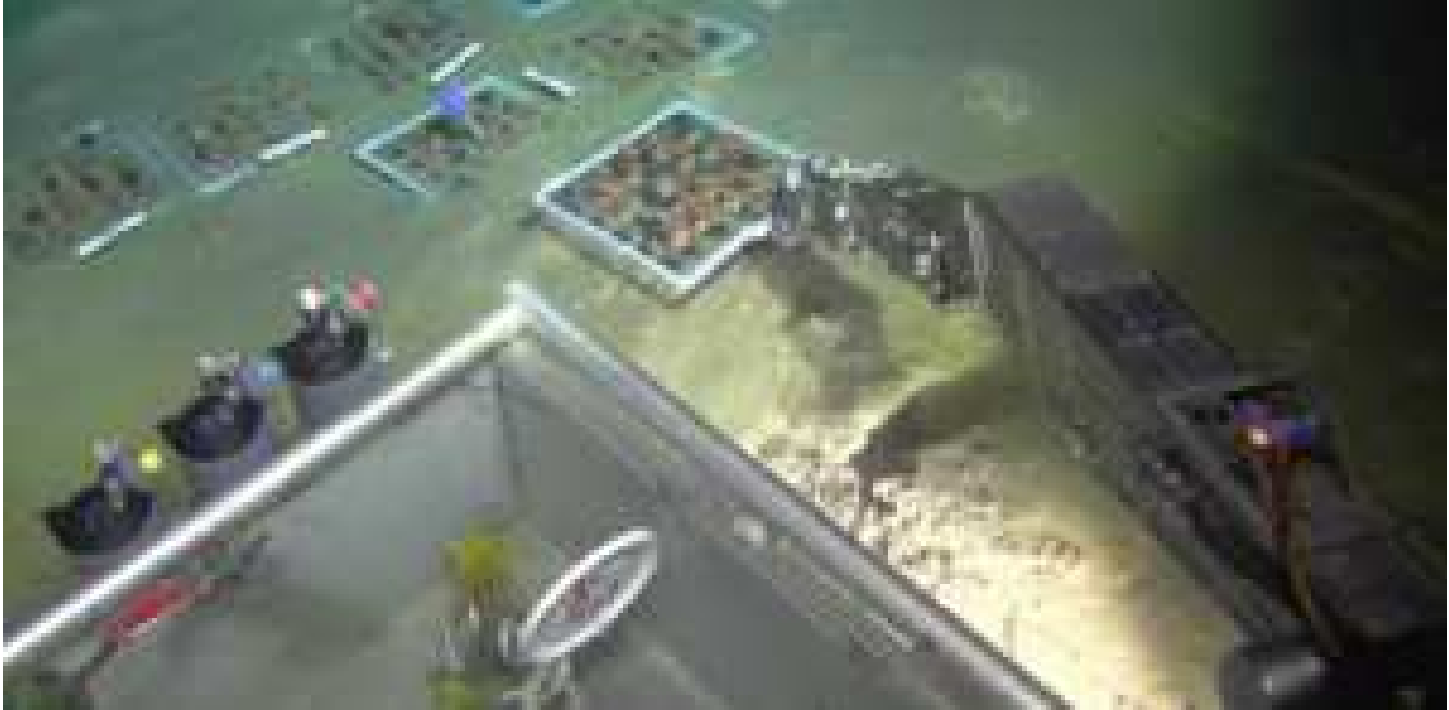
Figure 4.8: ROV manipulator arm deploying nodule frames on the seabed to conduct recolonization experiments. (Credit: MI2 & BGR)
