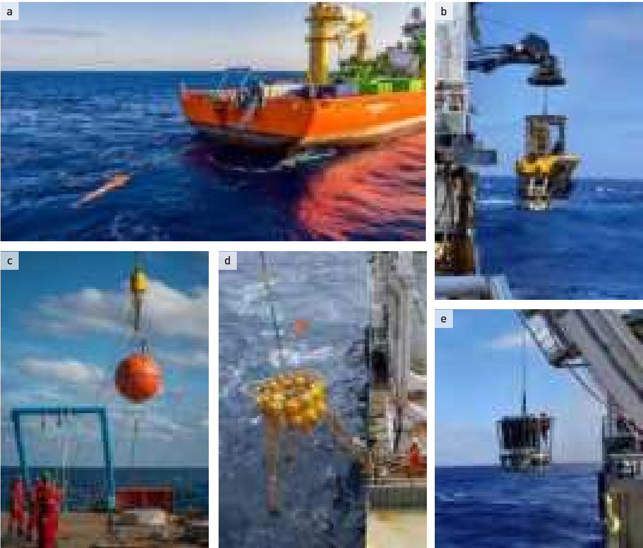
Figure 4.5: (a) HUGIN 6000 AUV off the stern of the MV Normand Energy . (b) Schilling ROV being deployed from the MV Island Pride . (Credit: MI2 & BGR) (c) A prepared mooring with flotation buoy (orange sphere) and concrete anchor, with a wire full of instrumentation in between, being raised above the deck of the MV Normand Energy . (d) The BoBo lander platform. (Credit: MI2 & BGR) (e) The CTD cage being deployed from the MV Island Pride . (Credit: MI2 & BGR)
