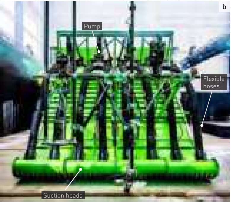
Figure 3.5: Side and front views of the Patania II pre-prototype collector vehicle. Key components indicated are the suction heads, flexible hoses for pumping water, pumps, rear diffuser, bucket, and tracks.
