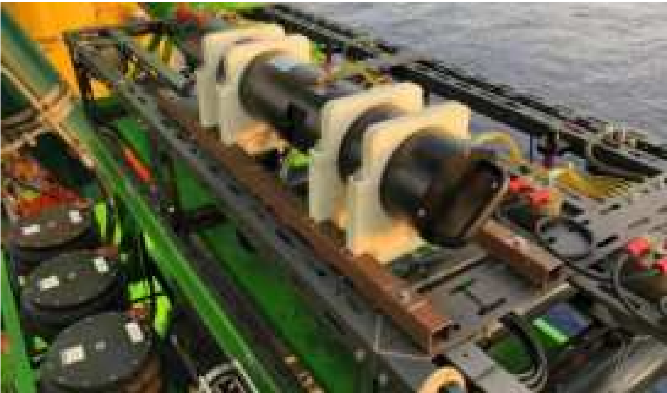
Figure 4.7: The RTSSV sensor mounted at the rear, atop the Patania II.
