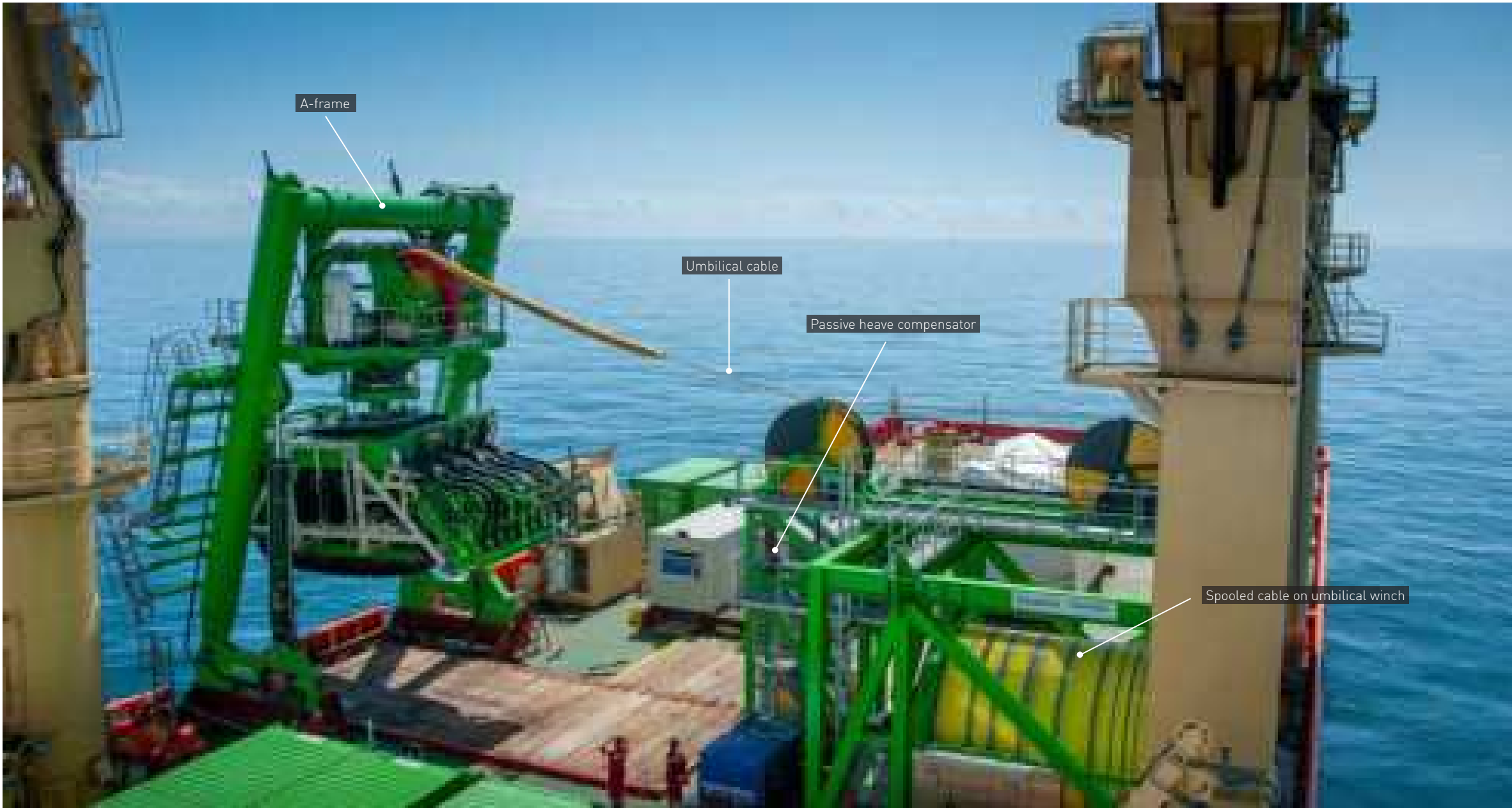
Figure 3.6: The redesigned Patania II LARS, including a passive heave compensator, being assessed during the GSRNOD19bis campaign in the Atlantic.
