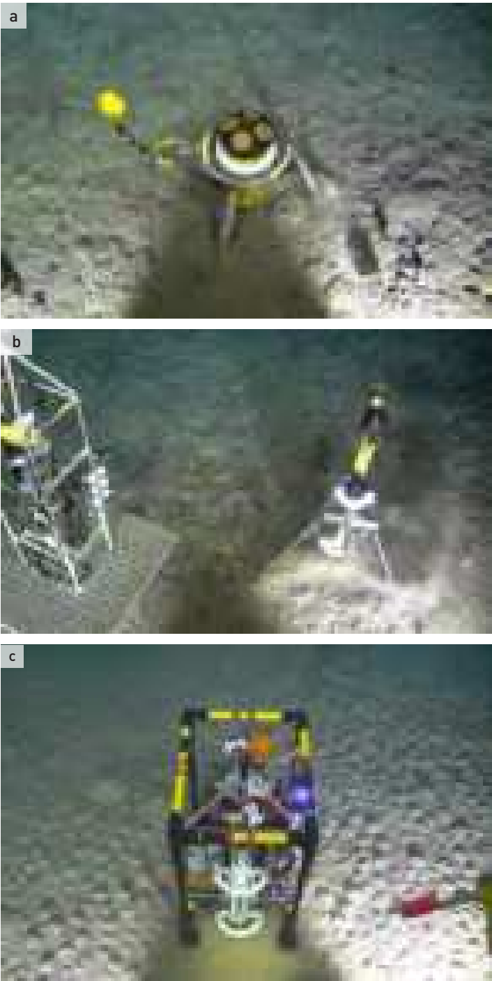
Figure 4.6: (a) An up-looking ADCP mounted in a bottom lander. (b) Two different bottom landers hosting a variety of equipment, including acoustic sensors, turbidity sensors and passive sampling membranes (the array of six white disks). (c) Seabed oxygen micro-profiler. (Credits: MI2 & BGR)
